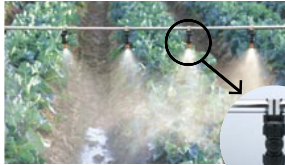
N-KS-8(KIRINASHI Nozzle) attached to a 2-Way Switchable Boom (KIRINASHI Nozzle head is recommended for those preferring minimal drift)
